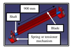
**Fig. 10** The proposed design of primary cleaner
