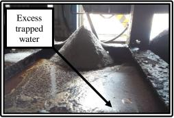
Excess trapped water due to the activity of cleaning up the conveyor belt by spraying water
