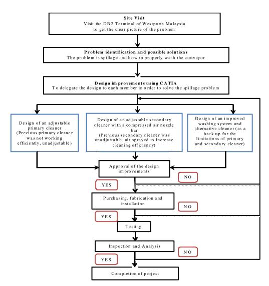
**Fig. 8** Flowchart of the design methodology
