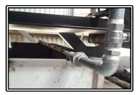
**Fig 20** Water spray bar
