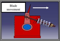
Close up view of the tensioner mechanism that is used to adjust the contact position of the blade with the pulley
